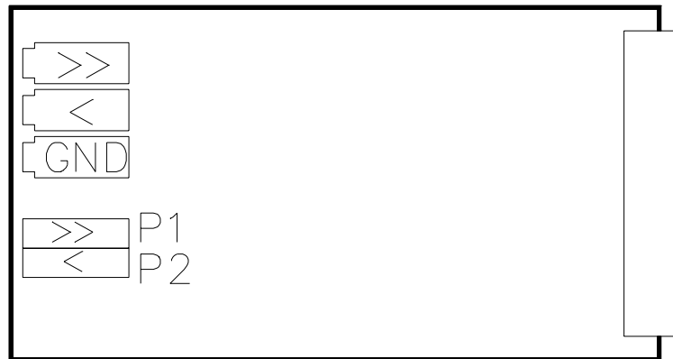
Fig. 7 - 1 The location of the potentiometers on the adaption board KL/KM 10202
